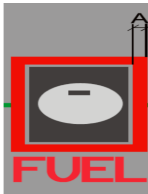
Gambar 5.2- 32 Marka Fuel Hydrant
