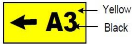
Gambar 5.4- 3 Runway exit sign
