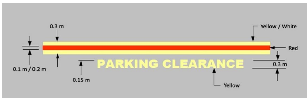
Gambar 5.2- 23 Parking Clearance Line
